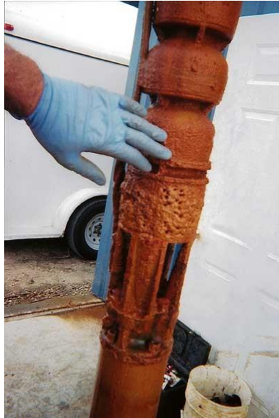
Figure 2-11 Iron bacteria on bowl assembly
