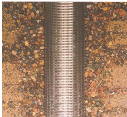
Figure 2-7 Properly developed natural packed screen well
