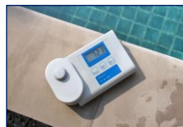
Figure 5-3 Chlorination Test equipment
